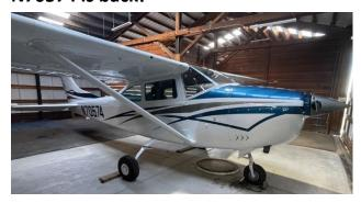
N70574 has returned from SunQuest Air Specialties at Paine Field (KPAE) and is absolutely stunning! In addition to being stripped and repainted, all the exterior fiberglass parts were replaced, the flaps were replaced (in addition to bearings and roller kit), the left elevator was replaced, the door and window seals were replaced, and a new cowl fastener kit was installed.
