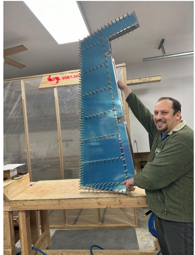
Me holding the rudder assembly. Note the makeshift priming paint booth in the background.
