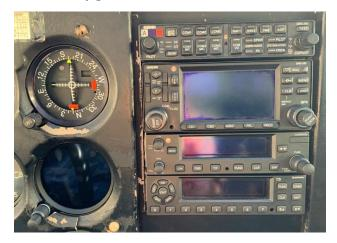
N5174E now has a new Garmin GNC 255A NAV/COM, a GI-275 CDI, and new COM coax cables installed. As previously noted, additional avionics upgrades are planned for 2024 to replace the audio panel and GNS 430 with new Garmin equipment.
