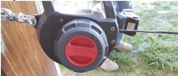
Rotate to the unlock position to pull the rope out; rotate to the locked position to engage the winch
