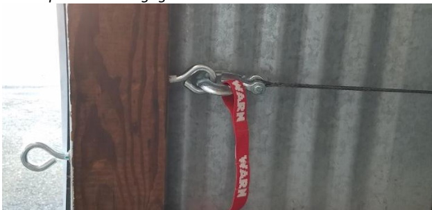
Connect to the eye bolt that is pointing in the direction that the winch is pulling
