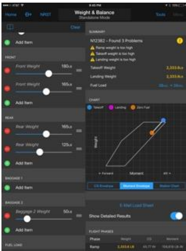
N12382 with a load outside its envelope
