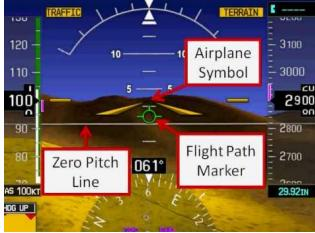
To enable synthetic vision, press the **PFD** soft key on the bottom right side of the PFD. This opens
