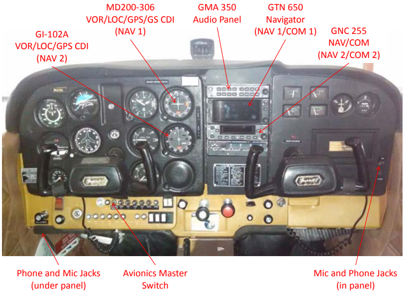
Figure 1: New Avionics in N12382.
